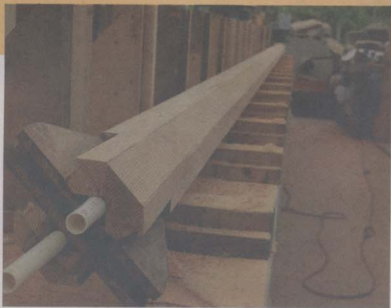
Here is the 32-foot mast after laminating but before final shaping to round. The first step in rounding a square mast is to cut it to 8 equal sides, then 16, then 32.
