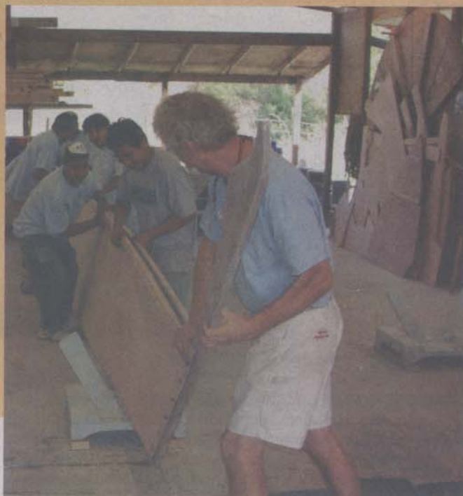
David Halladay and the Boatsmith crew getting the first hull set up. This photo illustrates the "stitch and glue" method of wiring plywood hull panels together prior to opening them up for inserting bulkheads.
